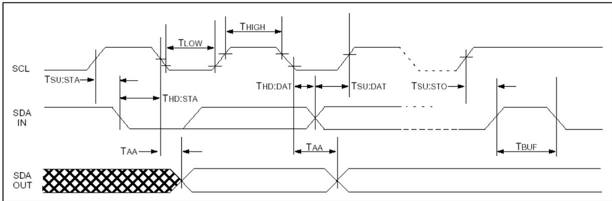
Figure 2.1 – I<sup>2</sup>C bus timing
