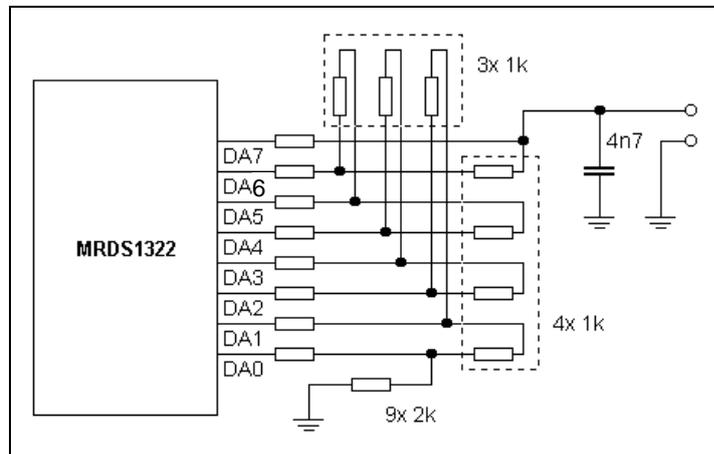
Figure 3.8 – 8-bit D/A converter R/2R network.
