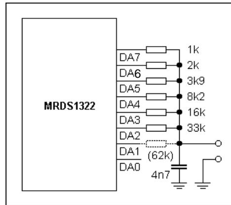
Figure 3.7 – 6 (or 7) -bit D/A converter network.
