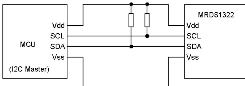
Figure 4.3 – Interfacing the MRDS1322 in mode 3.
