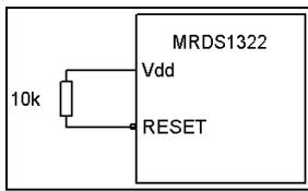
Figure 3.1 – Device reset.
