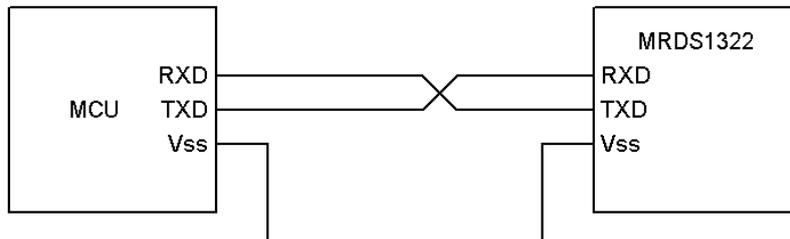
Figure 4.1 – Interfacing the MRDS1322 in mode 0 or 2.
