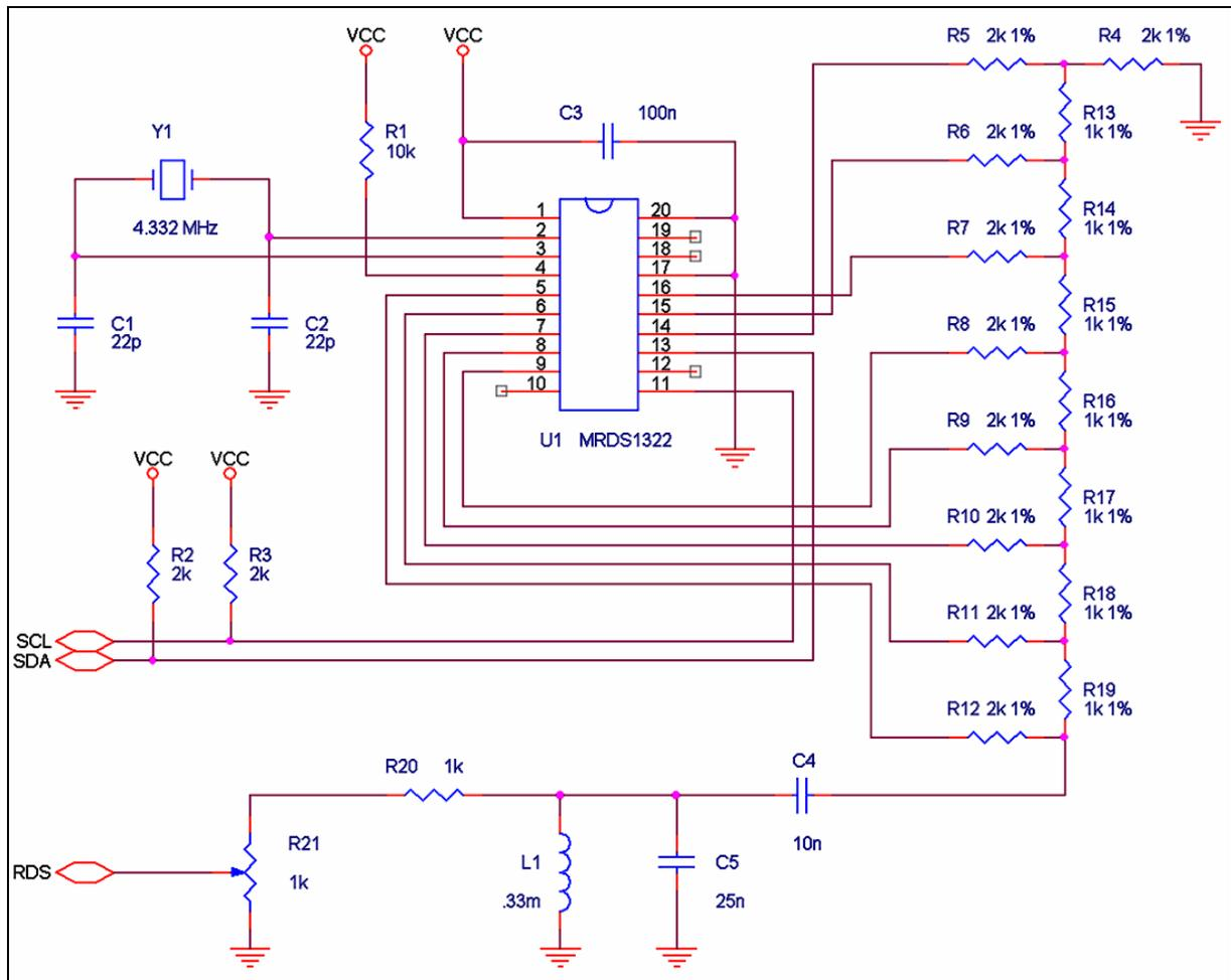
Figure 8.1 – Test circuit schematic diagram.
