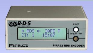
The PIRA32 RDS encoder meets requirements of most radio stations. Fully digital concept and uniquely effective design ensures high reliability, excellent signal characteristics and gives the user many advanced features. Includes scrolling, parsing, advanced weekly scheduling, EON, RT+, UECP, ASCII terminal control, front panel LCD and much more! Supported by all popular broadcast automation systems.
